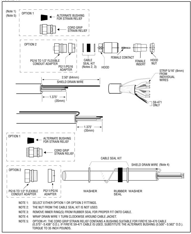
Note: Refer to Figures 19, 20, and 21 for proper wiring of the scanner cable to the appropriate controls.
