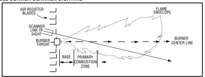
4. Consideration must be given to burner secondary air rotation (some burners have clockwise air rotation and others have counterclockwise). If combustion air enters the furnace with a rotational movement of sufficient velocity to deflect the ignitor flame in the direction of rotation, position the scanner 10 to 30 degrees downstream of the ignitor as shown in Figure 5 and close to the periphery of the burner throat (See Figure 4).
