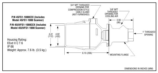
The "CEX" housing has a European approval (CENELEC) suitable for use in hazardous areas which include hydrogen gas.
