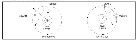
**5.** Having determined the approximate location for the sight pipe, cut a clearance hole for a 2 inch pipe through the burner plate. Look through the hole. If register vanes interfere with the desired line of sight, the interfering vane(s) should be trimmed to assure an unrestricted viewing path at all firing levels.
