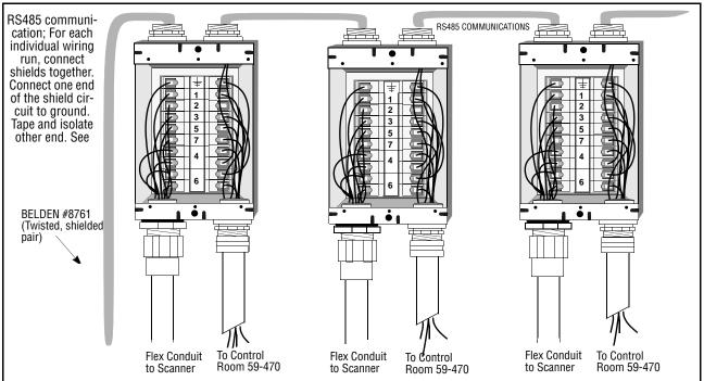
FIGURE 16. WIRING DIAGRAM FOR WIRING HARNESS
