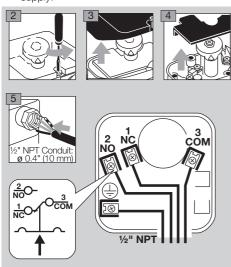
C6097A: the NO-to-COM connection is interrupted if the pressure drops (contacts 3 and 2 open).
