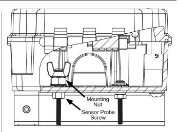
**Fig. 5:** Leak Detector with Attached Sensor (Attached sensor can also be mounted to a drip pan rim using the provided 7/64" hex set screws as shown above.)
