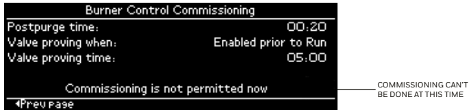
Fig. 66. Commissioning not permitted
