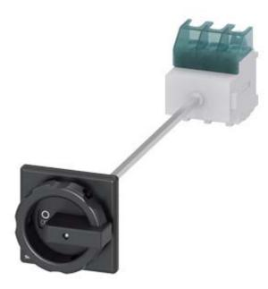
SENTRON, Switch disconnector 3LD, main switch, 3-pole, Iu: 63 A, Operating power / at AC-23 A at 400 V: 22 kW, floor mounting with door coupling, rotary operating mechanism, black, 4-hole mounting of the handle
