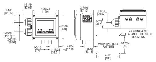
The **SERIES DHII** takes all the fabulous features of the standard Digihelic® Pressure Controller and packages them in a robust NEMA 4 (IP66) housing.
